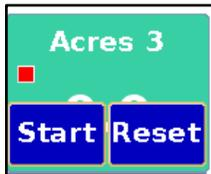
The acre counters will start counting anytime product is being applied in a section. Each section will stop counting anytime product is not being applied in that section. A lift switch can also be used to aid accurate area calculation.
